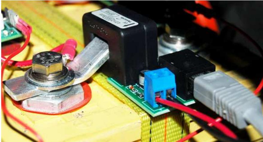
Once the sender unit is installed, connect 12V nominal power to the blue terminal on the sender unit. Watch for correct polarity. 12V power circuit must be always on, regardless of key switch position, since EV Display requires constant power source to keep track of battery SOC. You can power the unit from 12V aux battery or via DC-DC converter from the main pack, as long as DC-DC output is less than 15V and more than 10V.
